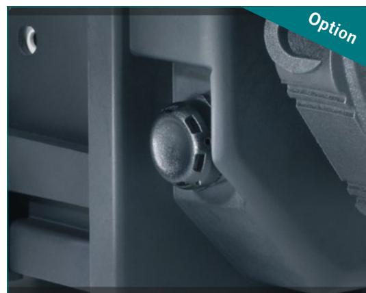
Long-life: The WISKA VentPLUG pressure compensation unit ensures constant pressure equalization between the interior and exterior and thus, minimizes the risk of condensation water
