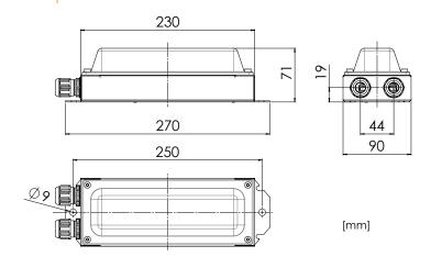
Stainless steel housing for outdoor marine environment Emergency battery back-up Different cable glands on request
